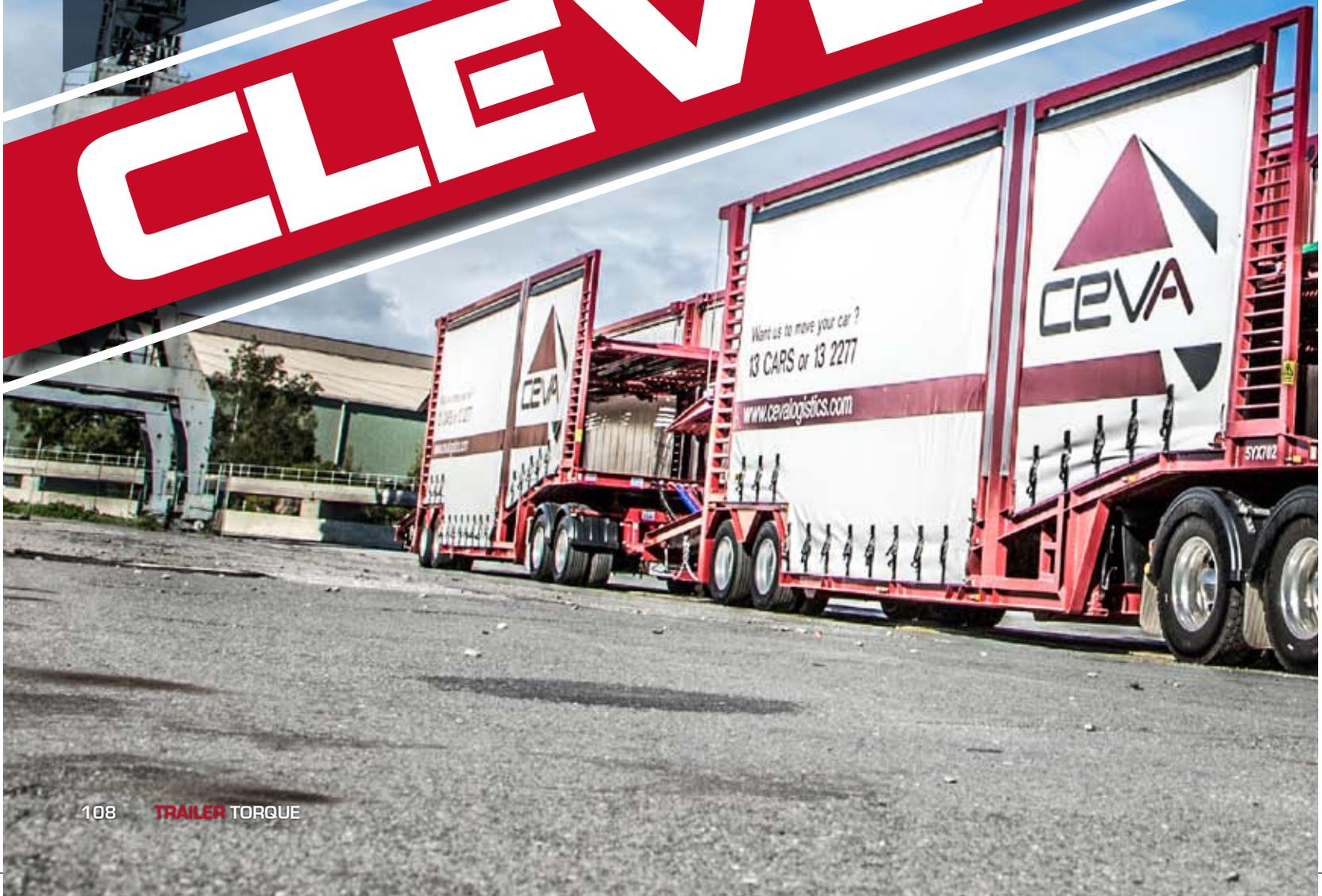
The new two-trailer road train combination operated by Kevin Schembri features the Transmech RTV2 design with each trailer being 45 ft (13.7 metres) in length and fitted with curtain side in-fill sections. The top decks are fully floating, as are the well decks, and these are moved into position through cables running on Nylatron sheaves. All locking bars are air operated.
